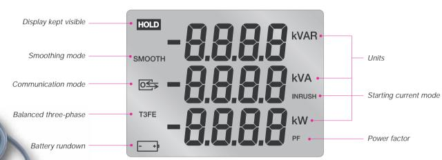
With the 73 x 54.3 mm LCD display, the user knows what the situation is at a glance. The battery rundown indicator light warns him when the period of autonomy is down to one hour.
