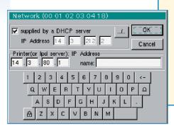
It is really simple to configure communications because, in most cases, the instrument's IP address is supplied automatically by the local server. All you have to do is enter the address of the printer to be used.
