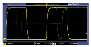
Discover – A waveform capture rate of 5,000 wfm/s maximizes the probability of capturing elusive glitches and other infrequent events.
