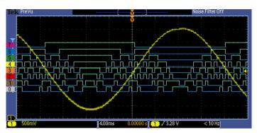
The MSO Series provides 16 integrated digital channels enabling you to view and analyze time-correlated analog and digital signals.
