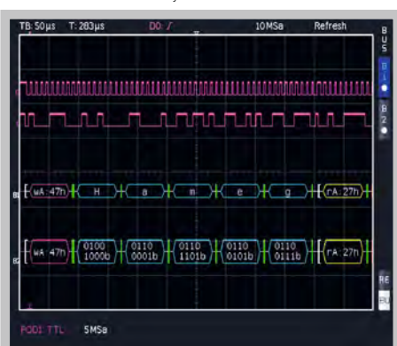
I 2 C Bus ASCII and binary
