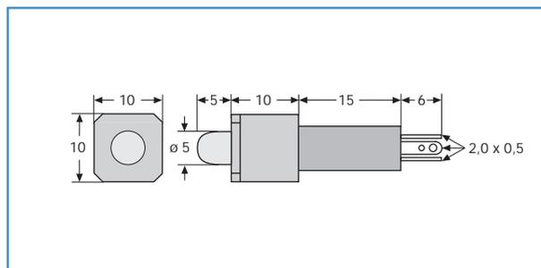
Alle angegebenen Maße in mm / All dimensions are given in mm
