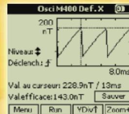
The C.A 42 also represents the variations of the electric or magnetic fields vs. time (oscilloscope function), or the harmonic and non-harmonic frequency distribution by calculation of the FFT.
