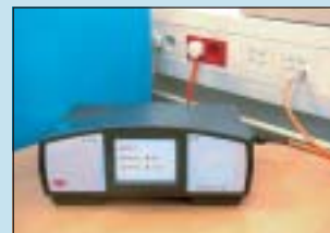
Certification of Cat 6 installations. Performance tests of all installations up to 350 MHz.
